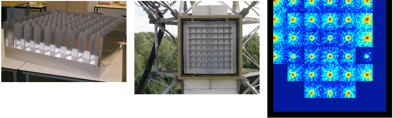
Figure 1: left: The array of 8x7x2 Vivaldi elements used for the prototype currently installed in RT5. middle: The same array installed in the focus of RT5. right: Beam patterns on the sky of a subset of the elements of the prototype. Each panel covers 3x3 degrees. The large optical distortions of the elements near the edge of the array can clearly be seen. Making compound beams by combining these element patterns will reduce these distortions.
