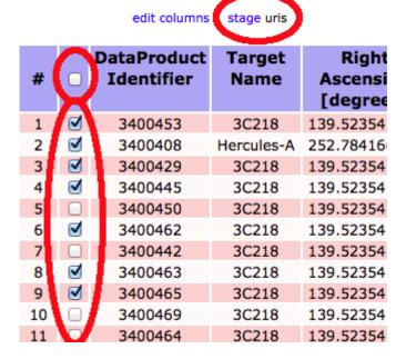
The LOFAR Archive stores data on magnetic tape. This means, that it cannot be downloaded right away, but has to be copied from tape to disk first. This process is called 'staging'.
